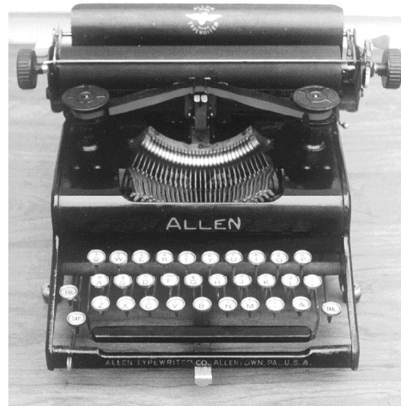
TOP: Allen 3-bank's first edition. Notice the name on the front, no type-basket cutout, small ribbon spools.
