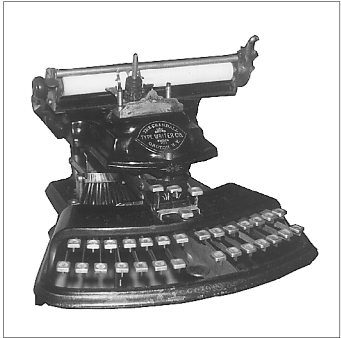
A rare early Crandall. Note the metal-framed keytops and metal space key. The machine features a more primitive paper feed device than later models as well as difference in ornamentation.
