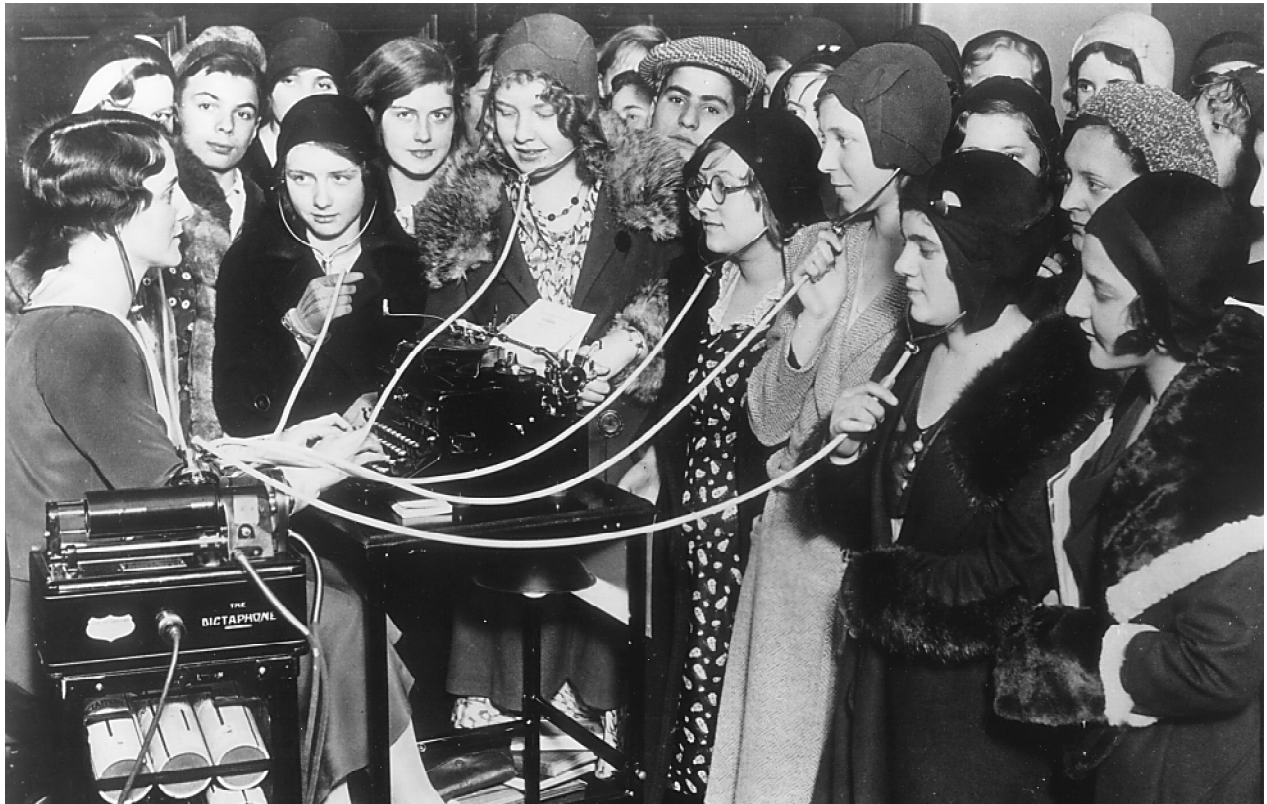
Dictaphone with a 6-way tube being demonstrated at a 1920's trade show. Photo provided by the Dictaphone Corporation
