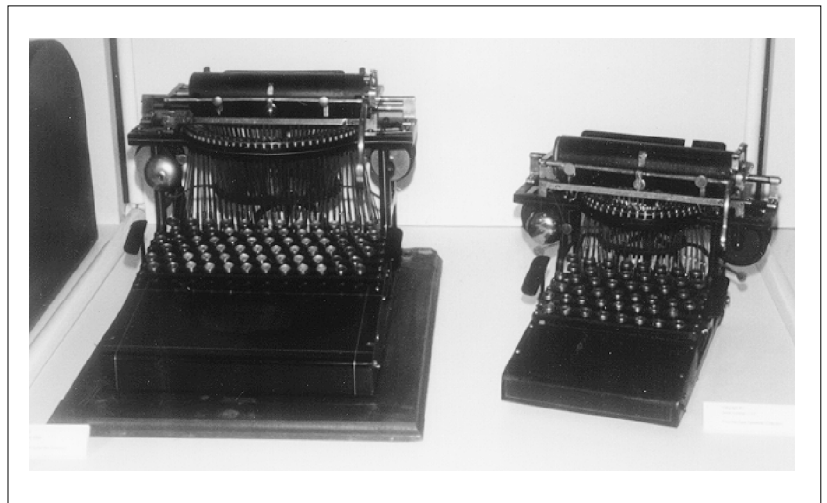
Only by seeing different Caligraphs side by side can you understand their difference in size. At left is the double-case Caligraph No. 2, and right, the diminutive caps-only Caligraph No. 1.
