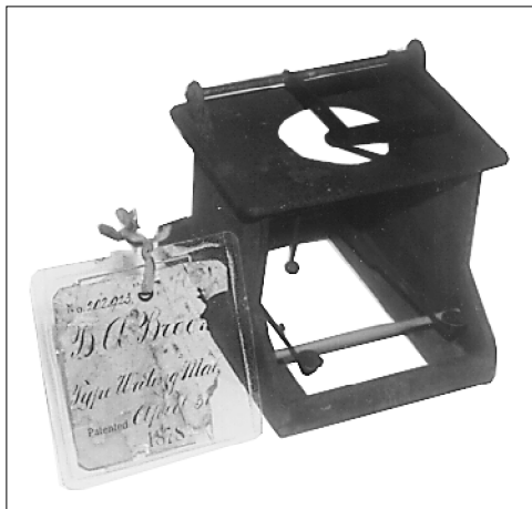
Another size surprise is the 1878 patent model submitted by Byron Brooks for the typewriter shift key. What may appear to be a full-size Sholes & Glidden frame is only a miniature, just 4" wide.
