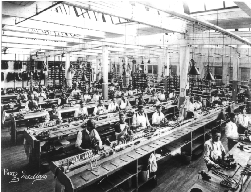
One of the assembly rooms at the Olivery factory in Woodstock, Illinois about 1909. Workmen are installing the famous U-shaped typebars.
